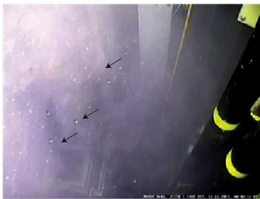
**Fig. 13.** Frame-grab photograph from drilling video of bubbles (black arrows) that were observed issuing from Hole M0070C and around the drill base during operations at this site, even when coring had stopped.
