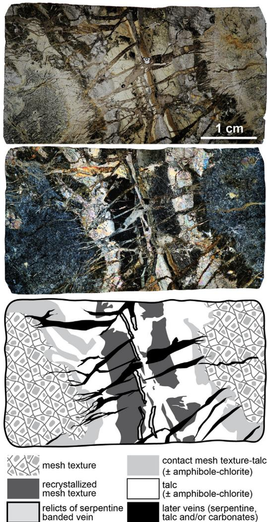
**Fig. 4.** Characteristic serpentine textures and cross-cutting relationships associated with progressive alteration and veining in serpentinized harzburgite (example from M0076B-7R1, 43–45 cm); (a) plane polarized light, (b) crossed polarized light, and (c) schematic representation of overprinting relationships. Modified from Früh-Green et al., 2017d, Fig. 7.
