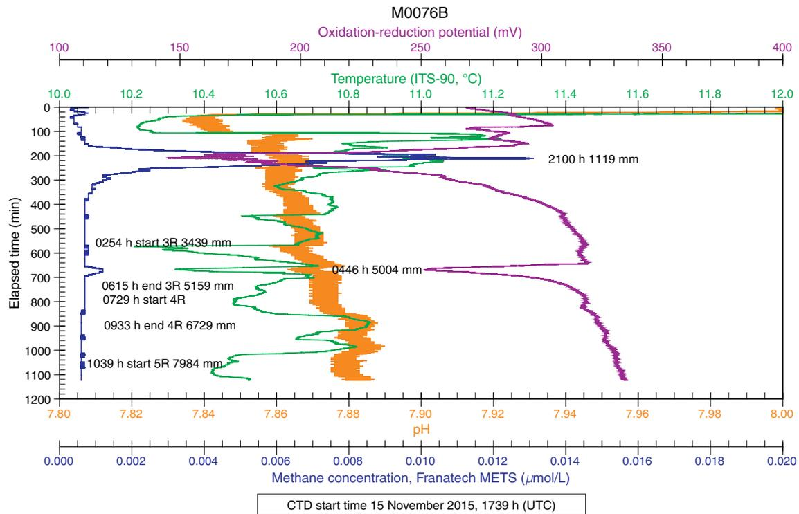
**Fig. 12.** Example of variations in fluid chemistry during drilling operations and correlations of geochemical signatures recorded by the sensor packages on the rock drills from sensor data for Hole M0076B, Cores 1R–5R. Elapsed time = time since the start of the sensor package data file. Penetration depth (in mm) was reconstructed from drill logs.
