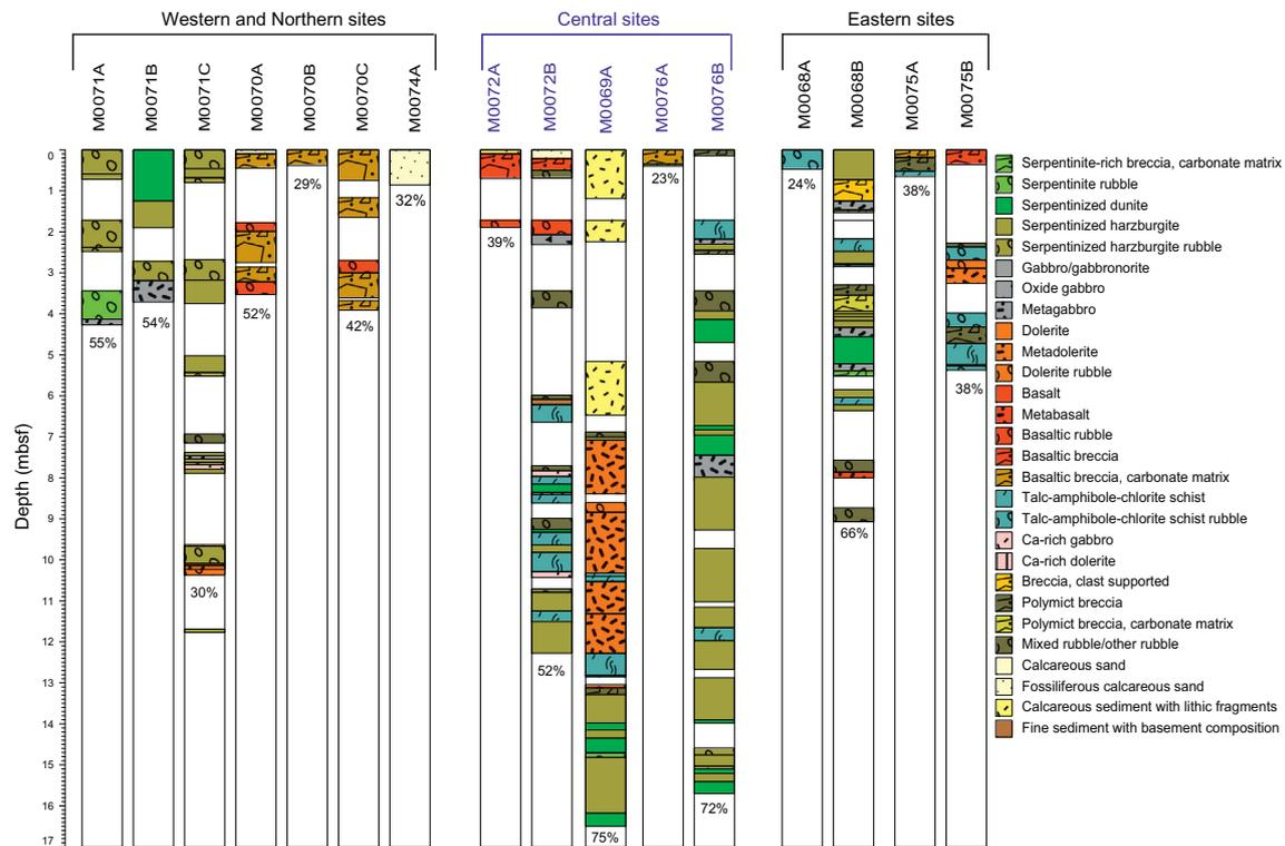
**Fig. 2.** Lithologic variations on a regional scale and with depth in cores recovered during IODP Expedition 357. Percentages indicate overall percent core recovery for each hole. The central sites, highlighted in blue, recovered in situ sequences, whereas talus debris was recovered at the western and eastern sites along the southern ridge.
